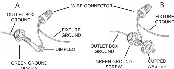
If fixture is provided with ground wire. Connect fixture ground wire to outlet box ground wire with wire connector, after following the above steps. Never connect ground wire to black or white power supply wires.
